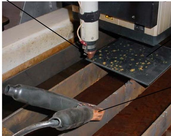
Place a piece of 12 gauge stock that is at least 6" X 6" on the material support slats.
