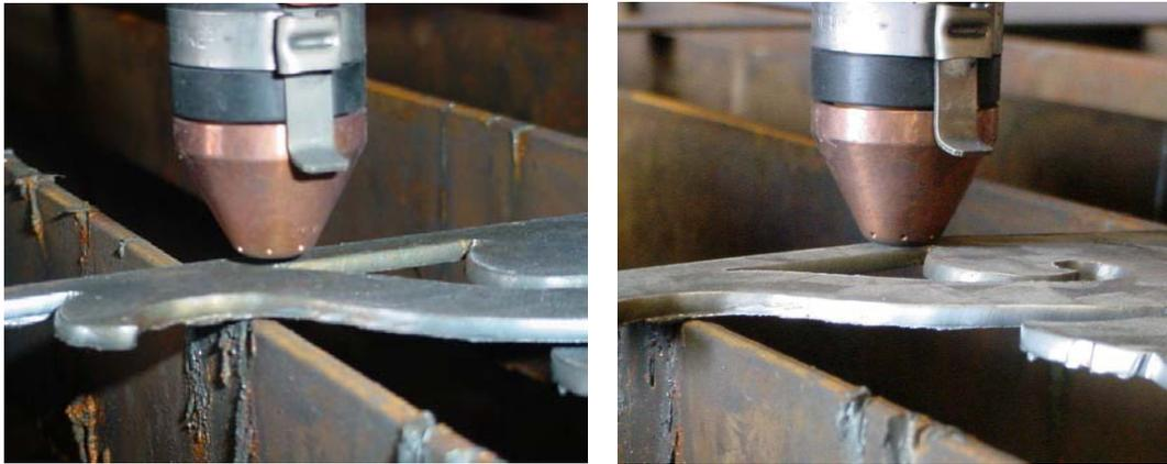
When a cut is started, the torch is held at the cut height. (left) If the metal heats up and warps up, the distance from the torch tip to the metal decreases. (right) This will result in a decrease in voltage. When the system senses this decrease in voltage, it will lift the torch up to compensate for the difference in voltage.
