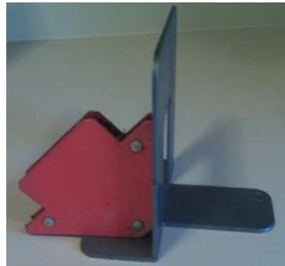
**Use a magnet to hold the parts at 90°.**
